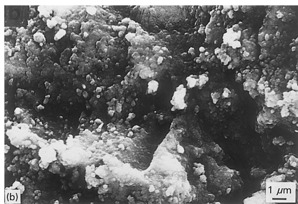
Figure 8 Scanning electron micrographs of \text{Pb}(\text{Mg}_{1/3}\text{Nb}_{2/3})\text{O}_3 powders prepared with different solvents: (a) ethanol-cyclohexane-acetone, (b) ethanol-cyclohexane.
